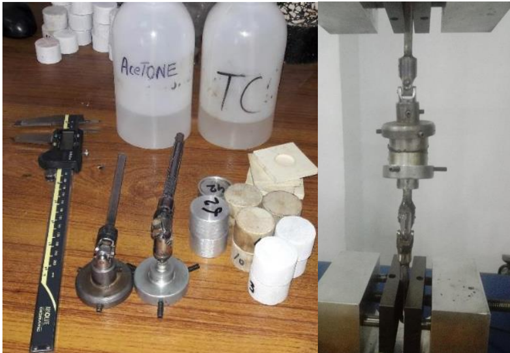
Figure 2: Direct pull-off testing assembly
