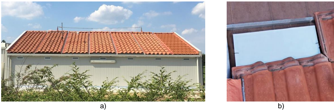
Figure 1: (a) Mock up building at the TekneHub Laboratory at the University of Ferrara; (b) Arrangement of the PCM plastic containers in the ASV layer of the roof.
