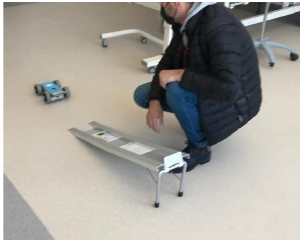
Figure 2: Surface slipperiness measuring process at a patient room with PVC vinyl floor.
