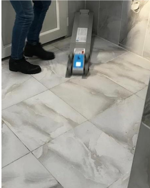
Figure 1: Surface slipperiness measuring process at a patient room toilet with ceramic tiles.
