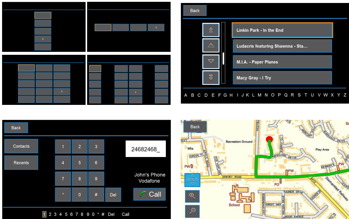
Figure 3. UK version of bespoke test interface used during study, showing (clockwise from top left): Menu Navigation, List Selection, Map Manipulation and Text Entry tasks.
