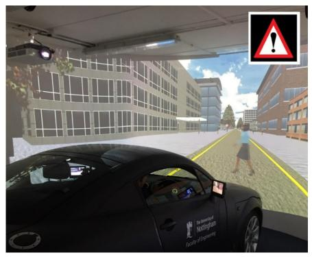
Figure 1: Driving simulator showing urban high-street scenario and pedestrian crossing road ahead, with visual alert icon that was presented on the HUD (inset).
