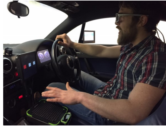
Figure 2. Participant interacting with mid-air haptics, showing transducer array (beneath hand), Leap Motion camera (beneath wrist) and visual (touchscreen) display with button 'one' of three selected (in red).
