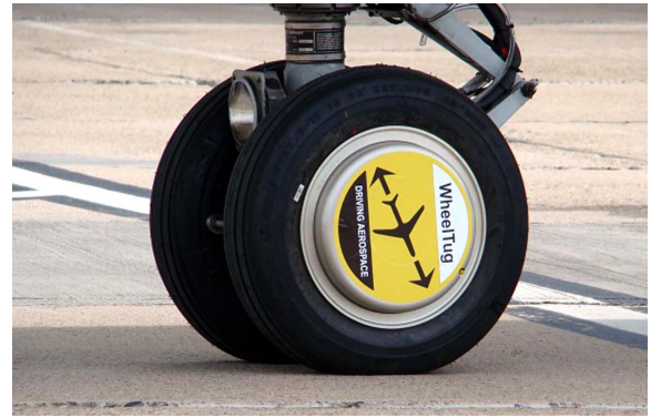
Fig. 2 WheelTug system implemented in NG
