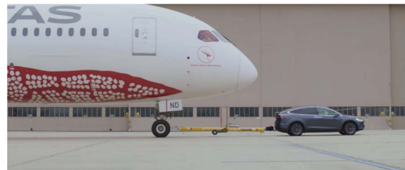
(a) Tesla-X towing the empty Boeing 787-9 with a mass of 130,000 kg.
