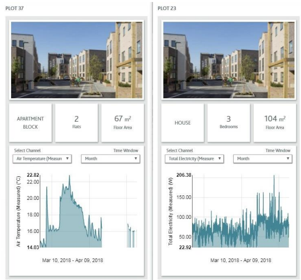
Figure 5: Examples of the dashboards of real-time data collection of the show apartment and show home.
