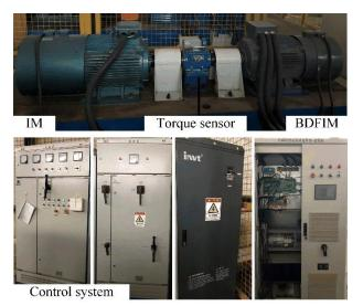
Fig. 11. The experimental platform.
