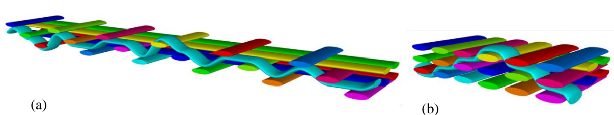
Figure 9. Angle interlock textile a) unconsolidated b) after consolidation
