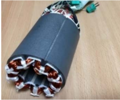
Fig. 4. Tested stator core and winding arrangement.
