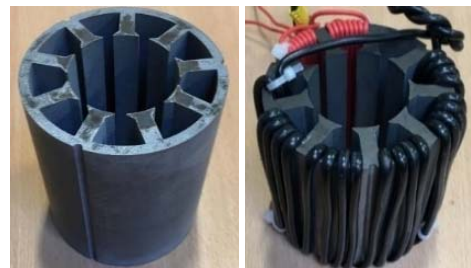
Fig. 7. Investigated stator core with and without measured coils.
