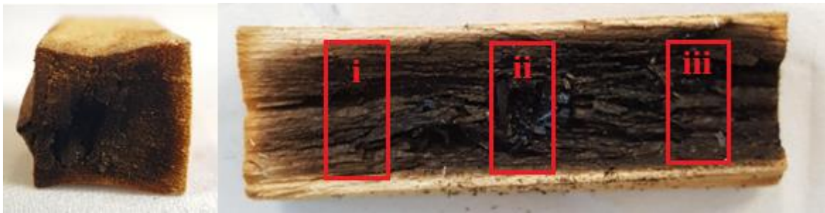
Figure 6 – Cross-sectional images of sycamore blocks after pyrolysis within n-hexane (45 x 15 x 15 mm).
