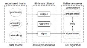
Fig. 1. The architecture of **libtissue**. Clients in **libtissue** monitor a host and provide input data to a **libtissue** server and AIS algorithm. Clients also allow algorithms to change the state of the monitored host.
