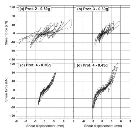
Fig. 11. Joint shear force versus the joint slip loops for an external beam-column joint (J13) of the third floor of: (a) Prototype 2 at PGA 0.30 g. (b) Prototype 3 at PGA 0.30 g. (c) Prototype 4 at PGA 0.30 g. (d) Prototype 4 at PGA 0.45 g.
