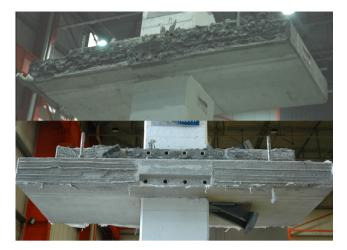
Fig. 14. Well executed and non satisfactory-filled joints as revealed at the demolition of the mock-up.
