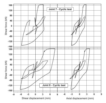
Fig. 12. Joint shear force versus joint slip and axial displacement recorded at the second floor of an external and a central joint during the cyclic test.
