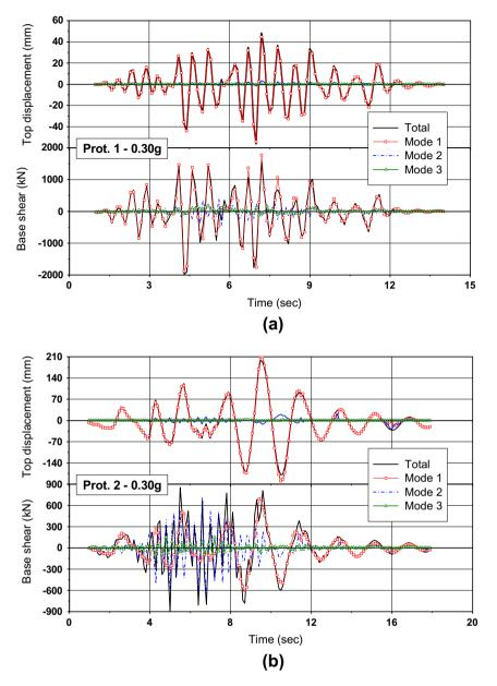
**Fig. 19.** Modal contribution response history of the 3-DoF system-in terms of roof displacement and base shear-to the applied ground motion of 0.30 g, for: (a) Prototype 1. (b) Prototype 2. (c) Prototype 3. (d) Prototype 4.
