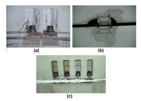
Fig. 17. Damages detected after the cyclic tests: (a) Cracking in the vicinity of the mechanical connector. (b) Broken slab-to-slab welded connections at the first floor.
