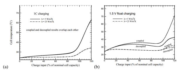
Figure 15: Comparison of predicted cell temperature between thermo-electrochemical coupled and decoupled model during (a) 1C charging and (b) 1.5V float charging [96].
