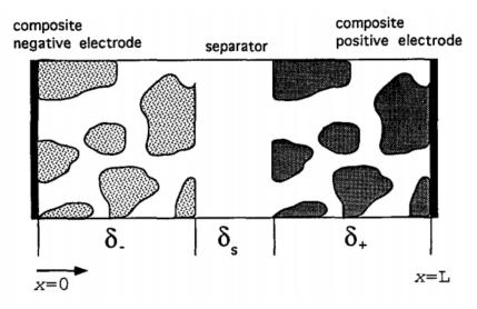
Figure 7: Dual lithium-ion insertion cell sandwich structure developed by [99].
