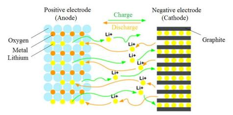
Figure 2: Lithium-ion battery mechanism during charge and discharge.
