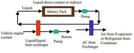
(c) Active liquid cooling/heating
