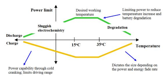
Figure 17: Temperature impact on life, safety and performance of lithium-ion batteries [138].
