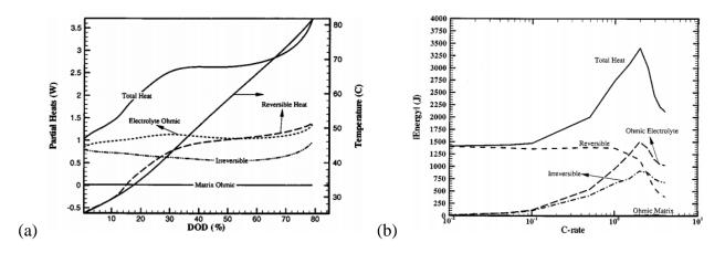
Figure 13: Heat generated due to various terms contributing to the total heat (a) under 2C discharge of a lithium-ion cell; and (b) under various discharge C rates [119].
