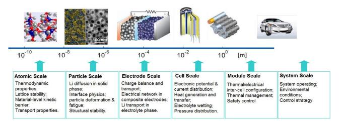
Figure 10: Multi-scale physics and micro-macroscopic modelling approach applied into a lithium-ion battery (modified from [109, 110]).
