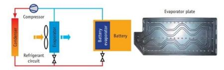
(a) Direct refrigerant-based cooling
