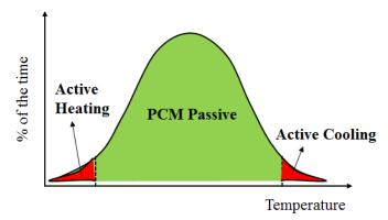
Figure 25: Hybrid air/PCM BTMS for EV normal operation
