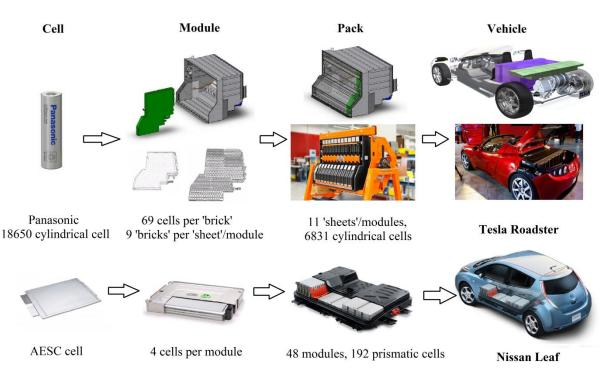
Figure 4: Lithium-ion battery cell-, module-, and pack-level demonstrated by two vehicle examples: Tesla Roadster [28, 29] and Nissan Leaf [30].
