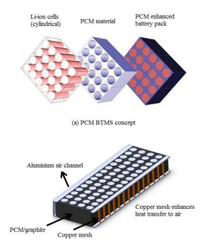
(b) AllCell hybrid air/PCM system design
