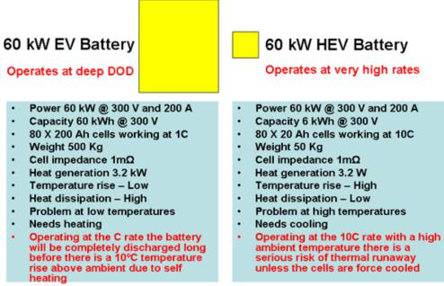
Figure 18: EV and HEV thermal & stress issues [146]
