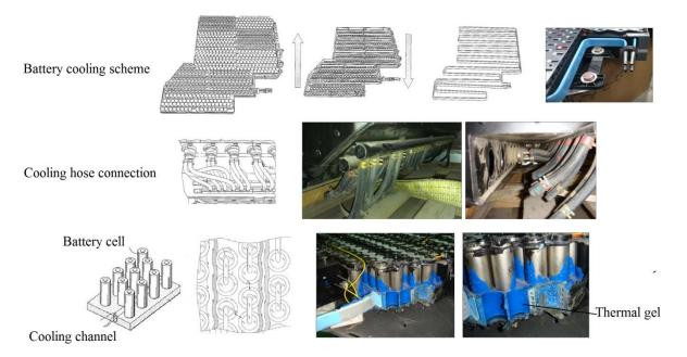
Figure 23: Tesla Roadster battery cooling (modified from [28, 62, 171, 172]).
