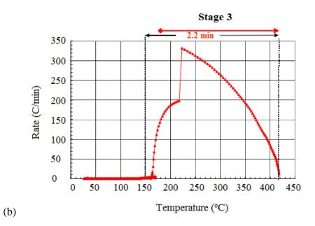
Figure 6: Illustrating three stages of the thermal response (thermal runaway path) obtained from SONY/GEN1/GEN2 lithium-ion cell [67]: (a) Stage 1-2 in scope; (b) Stage 3.
