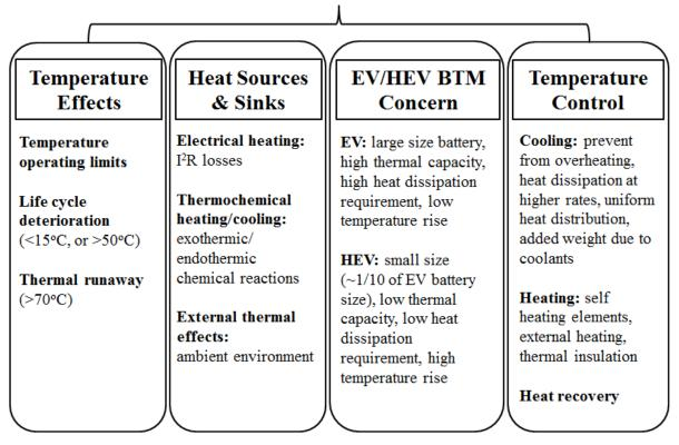
Figure 16: Battery thermal management mapping
