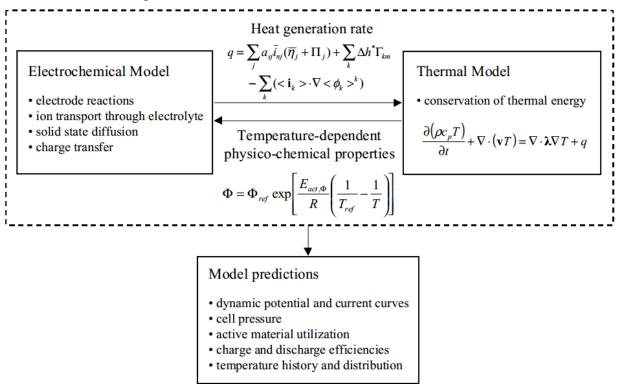
Figure 9: Thermal-electrochemical coupled modelling approach [96].
