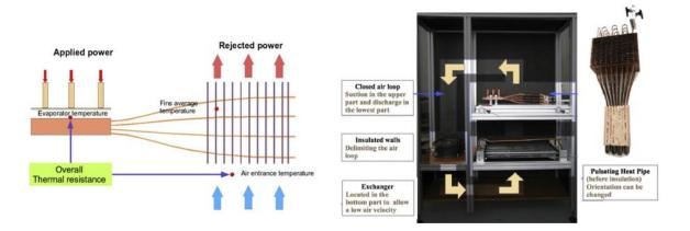
Figure 26: Pulsating heat pipe cooling a HEV lithium-ion battery pack [208].
