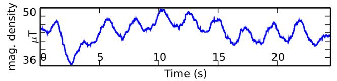
Fig. 5. Side to side rotation causes error in the recorded magnetic signal.
