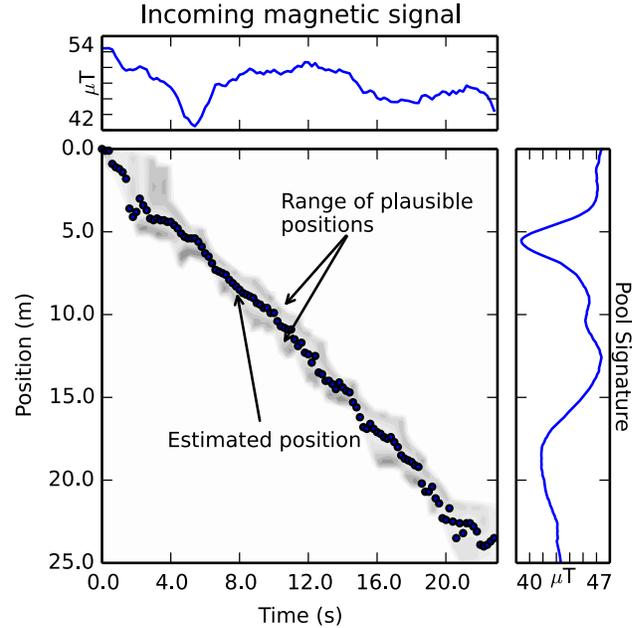
Fig. 8. A plot of a tracking result, showing the estimated position, and the range of positions which are plausible position estimates for each time step.
