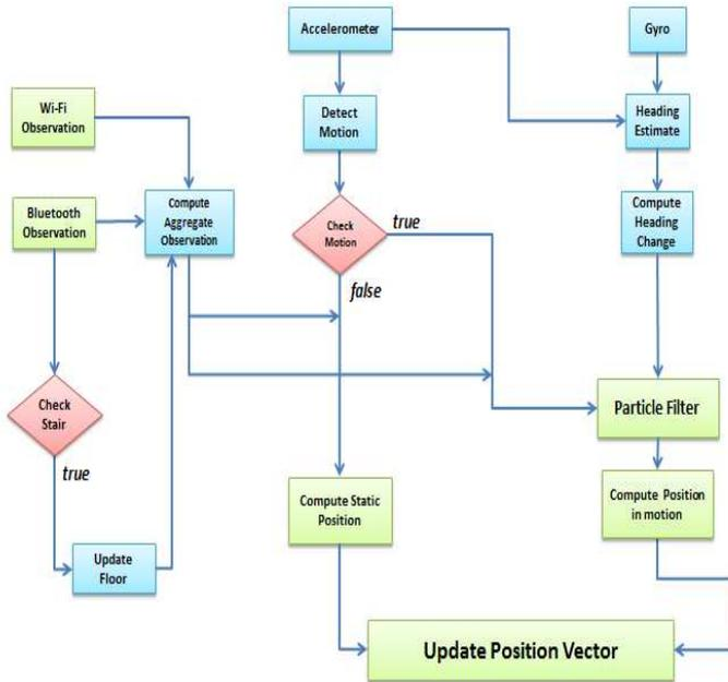
Fig. 15. Sensor fusion engine showing the different sensor integration
