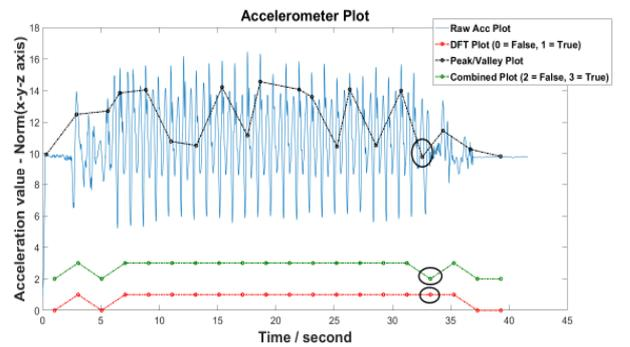
Fig. 6. Trial walk-2, circles showing wrongly detected motion in DFT but corrected using peak-valley analysis in the combined plot.
