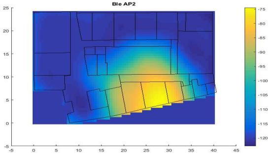
Fig. 12. BLE Heat map showing the signal variability.
