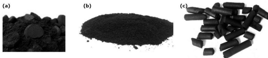
Fig. 1. SCG pellets manufacturing progression, (a) Raw SCG as received (moisture content greater than 60 wt%), (b) Dried SCG (moisture content  $\sim$  15 wt%), and (c) manufactured SCG pellets.
