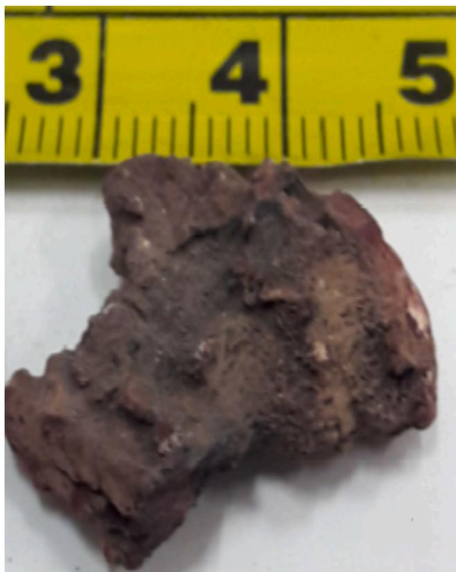
Fig. 12. Sample of agglomerates collected from the combustion of bituminous coal (BC) blended with wheat straw pellets (WS) at 40 wt% after 10 h of operation using silica sand as bed material (scale in cm). Picture from published work of the authors [49].
