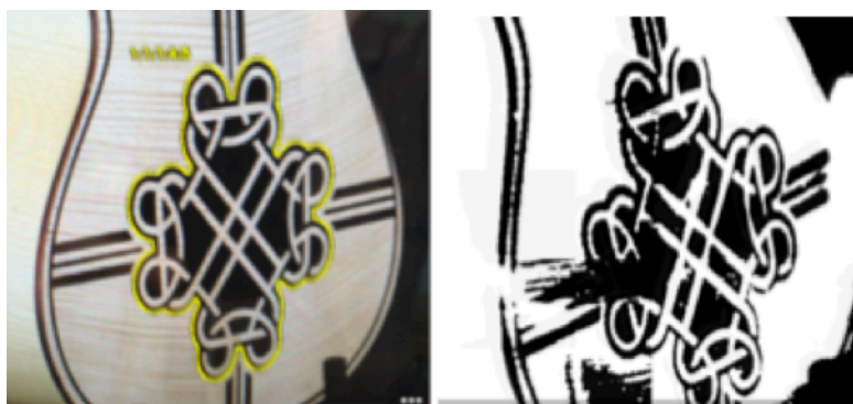
Figure 20. Two debug modes in the Artcodes app: showing the outlines of detected codes (left) and showing the image after thresholding (right)
