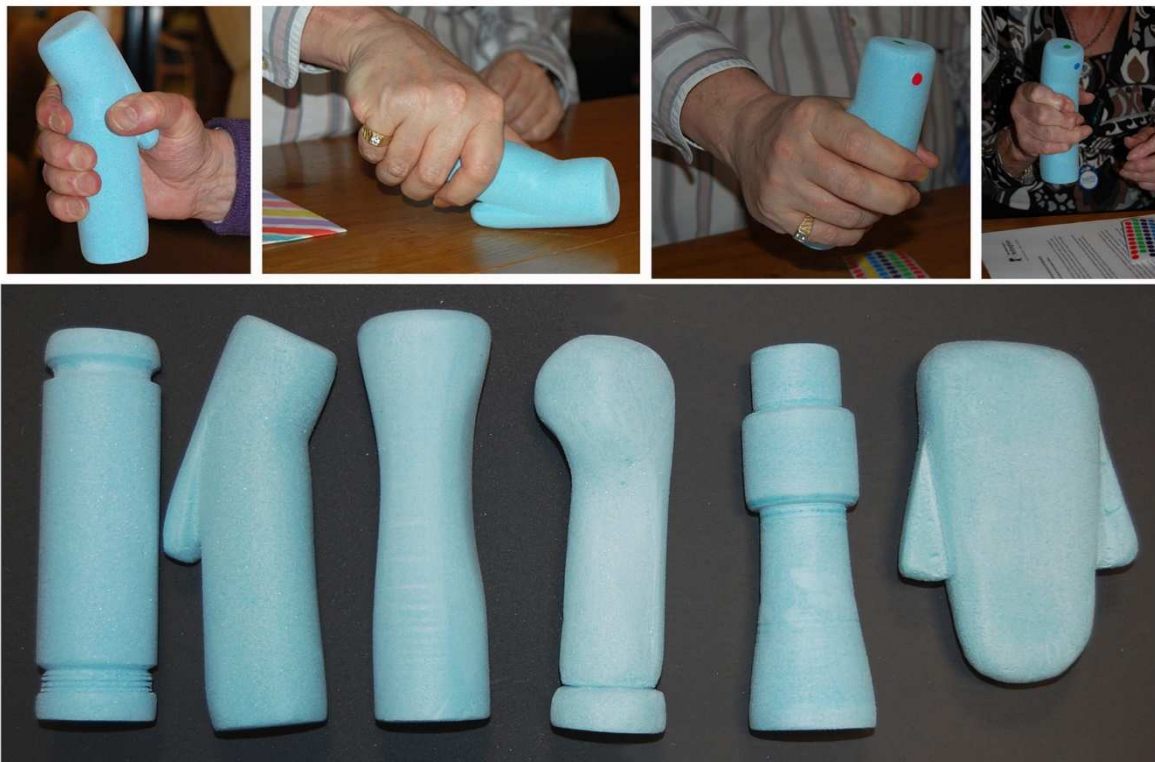
Figure 5. Focus Group- Participants were given the opportunity to hold and interact with Sketch models. The aim of this activity is to identify what forms are intuitive to hold and the best methods to activate the extinguisher.
