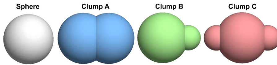
Fig. 1. Particle shapes used in DEM simulations.
