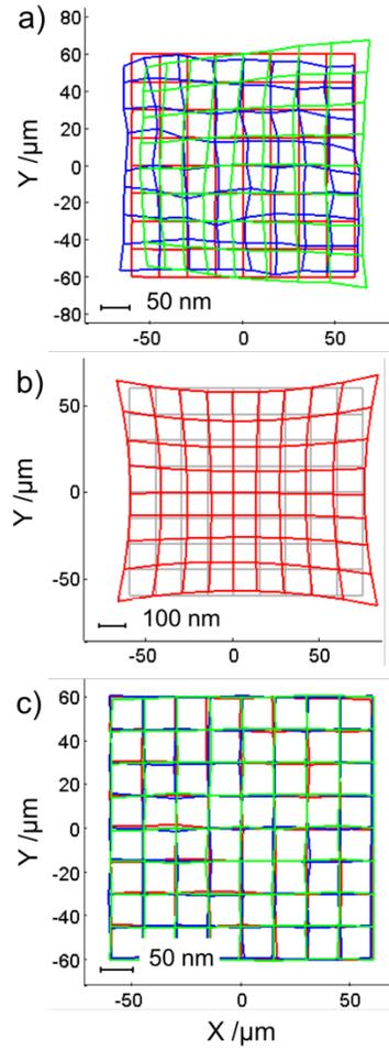
FIGURE 5. Self-calibration result. a) Input to the self-calibration algorithm and the placement scheme; b) calculated distortion of the CSI system with  $50\times$  magnification lens; c) overlay of the distortion-corrected grids.
