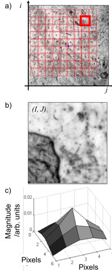
*FIGURE 2. Illustration of the image correlation method. a) A 9-by-9 grid of image patches defined in the 2D intensity map of the CSI measurement of a coin surface; b) the enlarged image patch (100-by-100 pixels) of which the centroid is located at  $(I, J)$  in the image coordinate; c) the correlation function which is the result of searching for the reference image patch around  $(I, J)$  in the translated or rotated views.*
