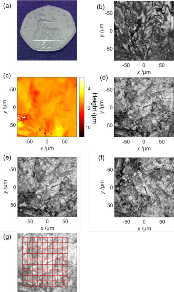
*FIGURE 3. Extraction of the 2D intensity maps from CSI measurements of a coin surface and definition of the grid. a) Picture of the coin; b) an image slice from the 3D fringe data; c) calculated height map; d, e, f) Intensity maps of the reference, translated and rotated views, respectively; g) defined grid and image patches. The grey scales of all intensity images are normalised. The 50 $\times$  objective lens was used.*
