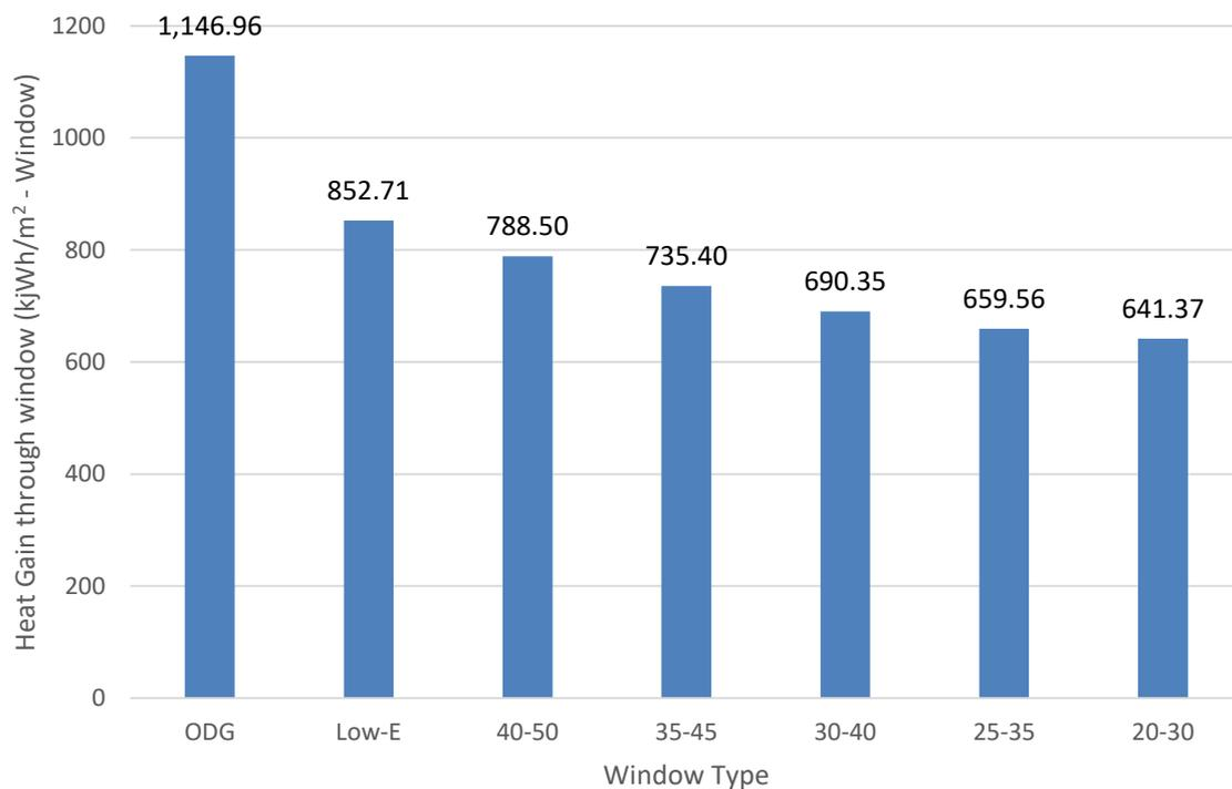
Figure 14 – Annual Window Total heat Gain comparison between the different windows and transition temperature ranges
