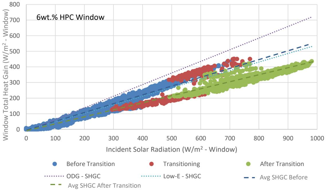
Figure 5 - Window Solar Heat Gain Coefficients for the 2, 4 and 6wt.% HPC Thermotropic (TT) Windows
