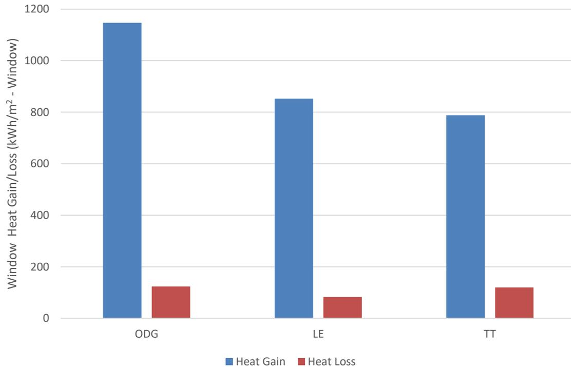
Figure 11 - Annual window heat gains/losses comparison between ODG, LE and 6% HPC TT
