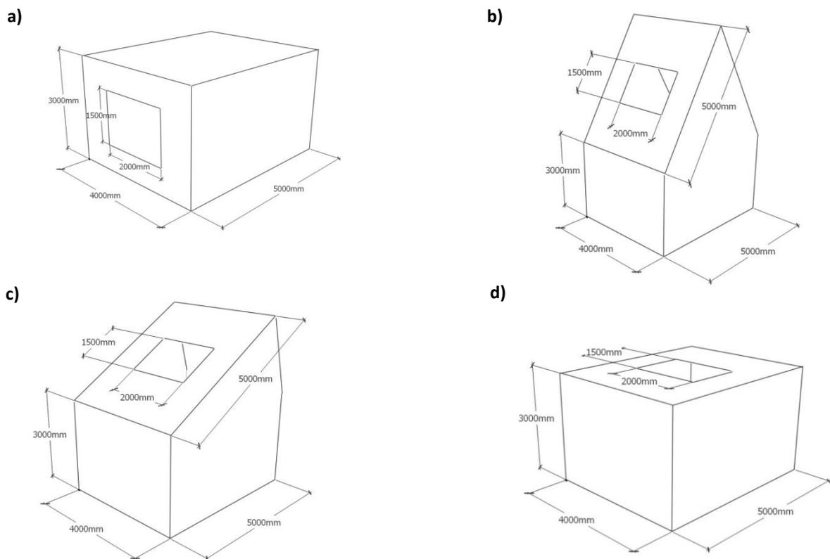
Figure 2 – Room simulations a) 90°, b) 60°, c) 30°, d) 0°, orientated window from horizontal
