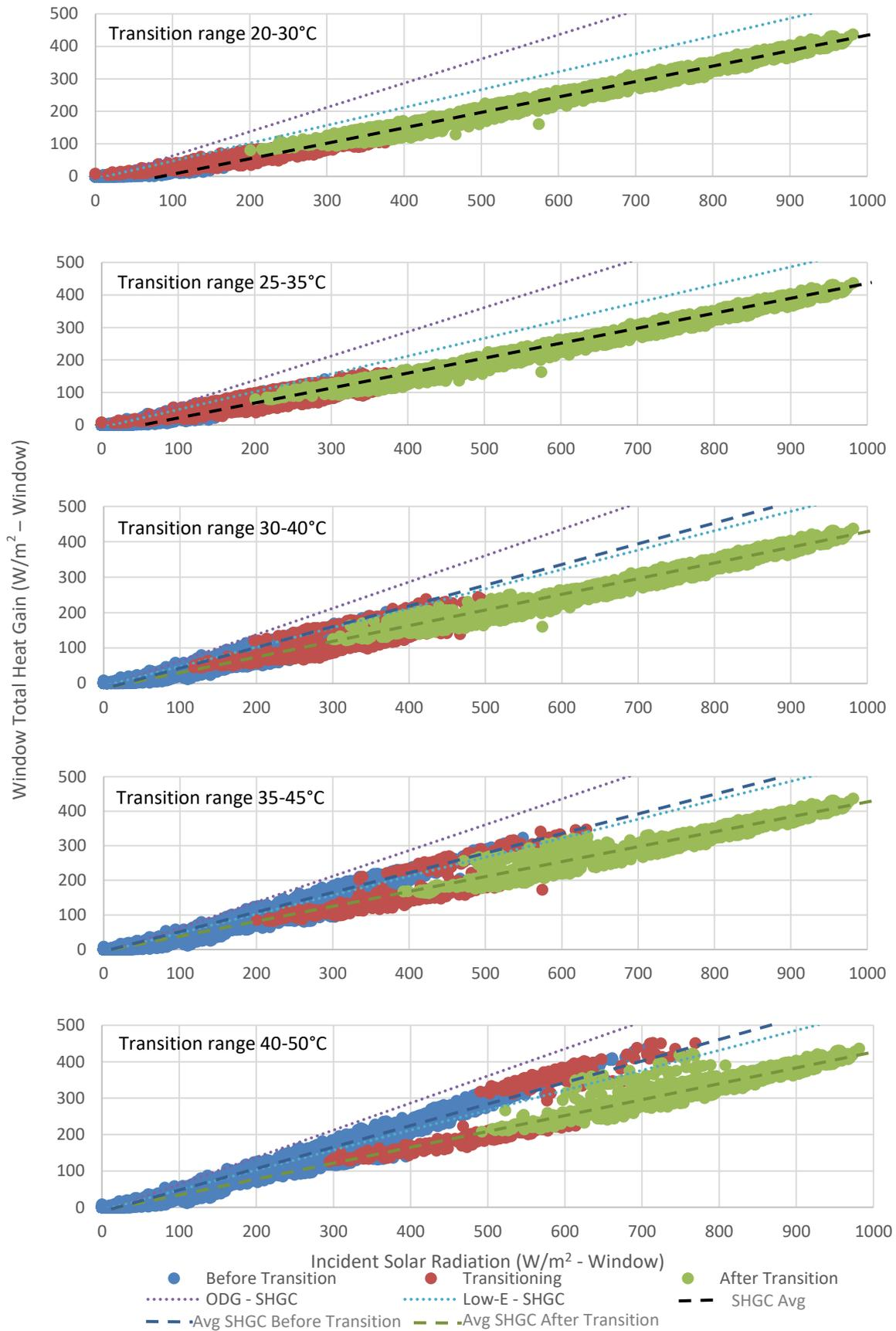
Figure 15 – Window Solar Heat Gain Coefficients for the different transition temperature ranges
