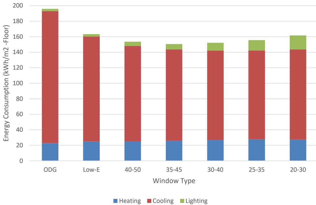
**Figure 16 – Annual Energy consumption comparison between the different types/transition temperature ranges**
