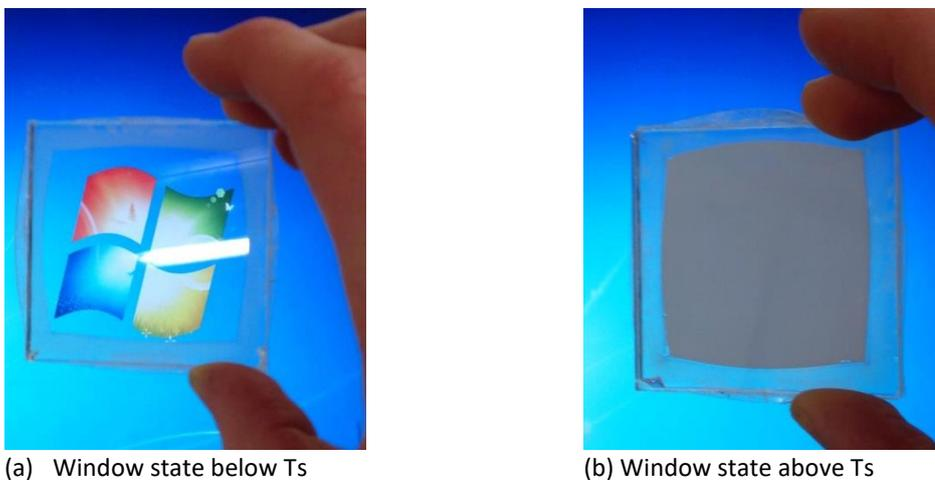
Figure 1 - Photo of the developed thermotropic smart window
