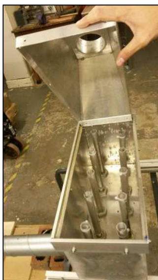
Figure 2 (a) Internal view of reactor showing perforated diffuser pipe allocation
