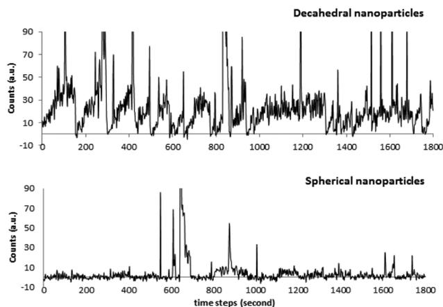
**Fig. 4** Raman bursts for the C–C band at  $1586\text{ cm}^{-1}$  from surface-adsorbed thiophenol on (a) a 36 nm decahedral silver nanoparticle and (b) a 40 nm spherical silver nanoparticle. Suspensions were made in Tris pH 7.4 buffer solution at the same concentration. Bursts are integrated over a 2 second interval. The number of counts measured for the maximum of the C–C symmetric peak is adjusted for background by subtracting the average readings from either side of the band feature.
