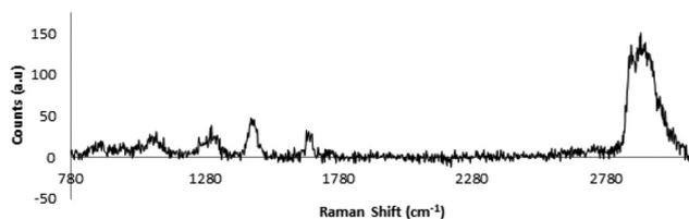
**Fig. 6** A Raman spectrum recorded for 2 seconds from an optically-trapped GUV with a diameter of approximately 5 μm showing five clear lipid peaks at 1094, 1317, 1458, 1672 and 2935 cm<sup>-1</sup>. A background signal has been subtracted.
