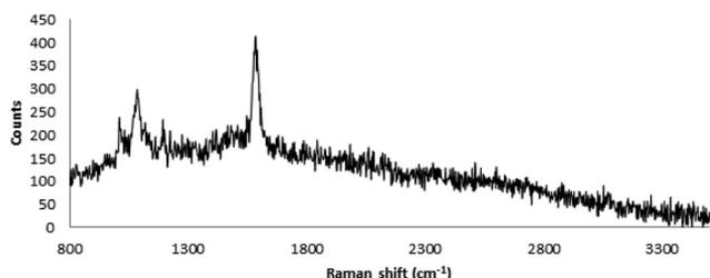
**Fig. 3** A SERS spectrum recorded from an optically-trapped 36 nm diameter decahedral nanoparticle with a monolayer coating of thiophenol. Spectral integration time is 2 seconds. The fluorescence-background has not been subtracted from the spectrum. The signal-to-noise-ratio is estimated to be  $\sim 16$ .
