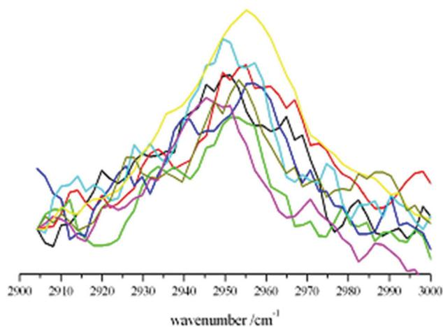
**Fig. 10** The main lipid peak for 8 overlapping example spectra recorded from 41 nm diameter decahedral nanoparticles encapsulated in 50 nm lipid vesicles. Each plot representing a different single vesicle made from the same lipid composition highlighting the reproducibility of the results.
