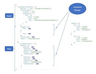
Fig. 3. Generic asset administration shell representation (left). Skill submodel is developed, submodel elements contains the skill API calls along with pertaining data that can be used by the client services. Component manager is deployed when the submodels are listed (right).
