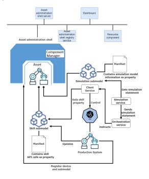
Fig. 6. Asset administration shell integration approach for testing processes. Control is guided through services, through Skill and Simulation submodels containing API calls and simulation data respectively
