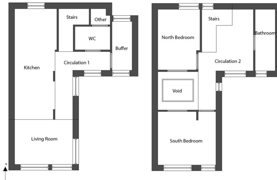
Figure 2. Ground floor (left) and first floor (right) plans and zones. Model created in EDSL Tas.
