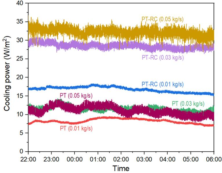
Fig. 10. The cooling power of the PT and PT-RC collectors during the radiative cooling mode with different air mass flow rates. Note: For the PT collector, the relative mean error of the cooling power is 6.0%, 12.0%, and 22.9% when the air mass flow rate is 0.01 kg/s, 0.03kg/s, and 0.05 kg/s, respectively; For the PT-RC collector, the relative mean error of the cooling power is 2.9%, 5.0%, and 6.8% when the air mass flow rate is 0.01 kg/s, 0.03kg/s, and 0.05 kg/s, respectively
