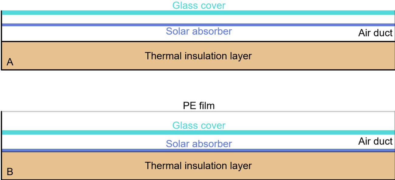
Fig. 1. The cross-section schematic diagram of the (A) typical solar air collector and (B) air-based PT-RC collector.
