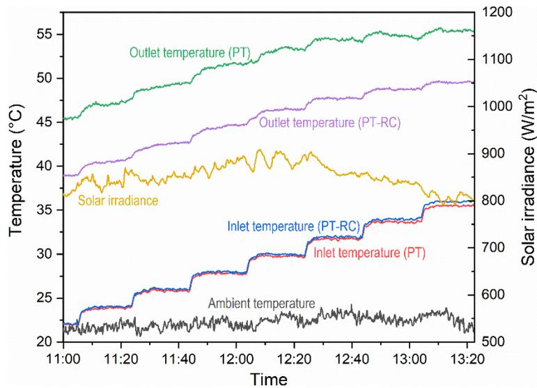
Fig. 5. The inlet and outlet temperature profiles of the PT and PT-RC collectors and the weather data during the solar heating mode with different inlet-ambient temperature differences.
