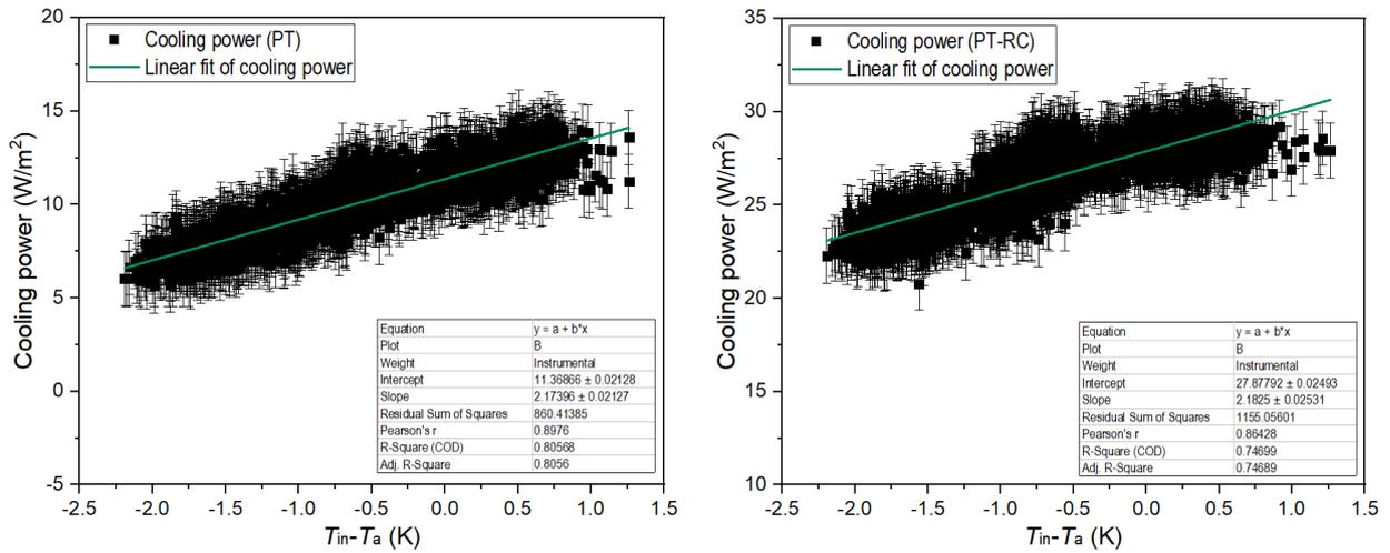
Fig. 8. The cooling power of the typical PT collector and air-based PT-RC collector at different inlet-ambient air temperature differences.
