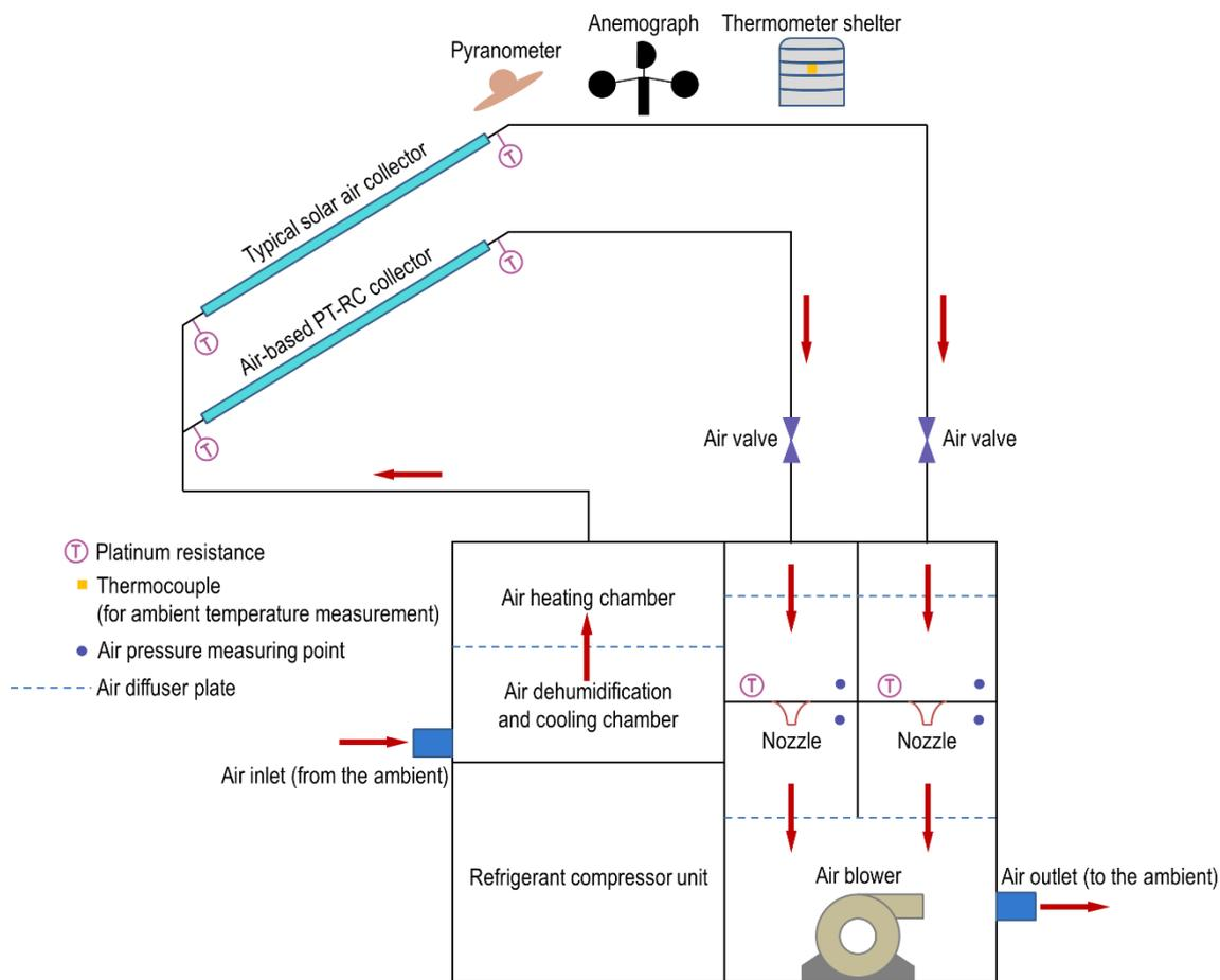
Fig. 2. Schematic of the experimental testing system.
