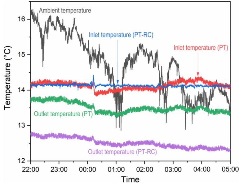
Fig. 7. The inlet and outlet temperature profiles of the PT and PT-RC collectors and the weather data during the radiative cooling mode with different inlet-ambient temperature differences.
