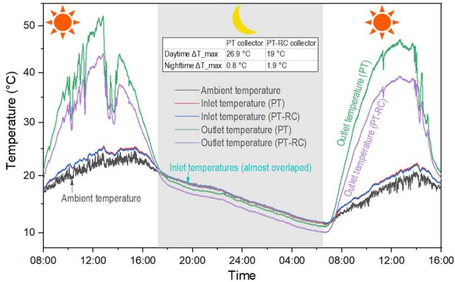
Fig. 4. Temperature profiles of the PT and PT-RC collectors over 32-hour consecutive testing. Note: offset reciprocal is applied on the vertical axis.
