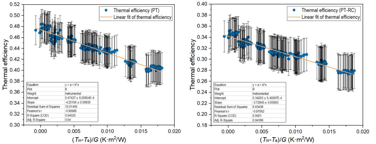
Fig. 6. The thermal efficiency of the typical PT collector and air-based PT-RC collector at different reduced temperatures.
