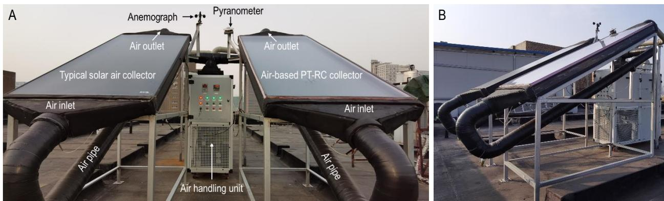
Fig. 3. In-situ photos of the experimental testing system. (A) front view, and (B) side view.
