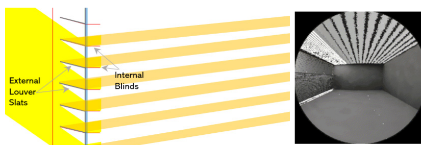
(b) Parametric louver attached with internal blinds.
