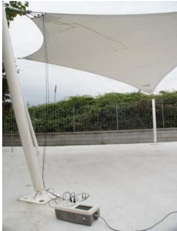
Fig. 8: Detail of the demonstrator for the calibration of the vibration sensors .
