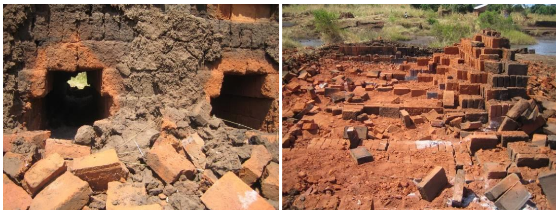
Figure 133: High material waste during production and handling (Tanzania).
