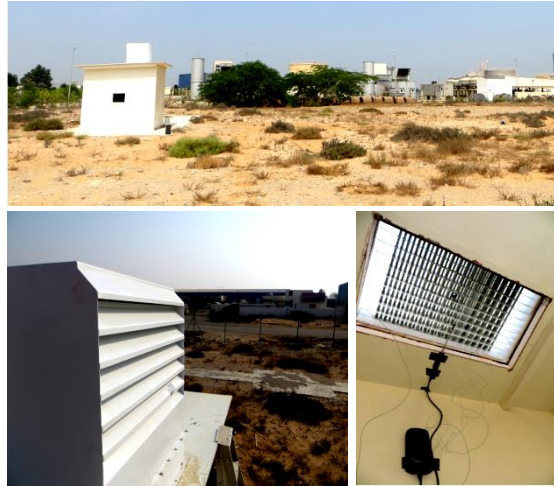
Figure 6: Test site in Ras Al-Khaimah (top) wind catcher mounted on the roof (bottom left) measurement setup (bottom right).
