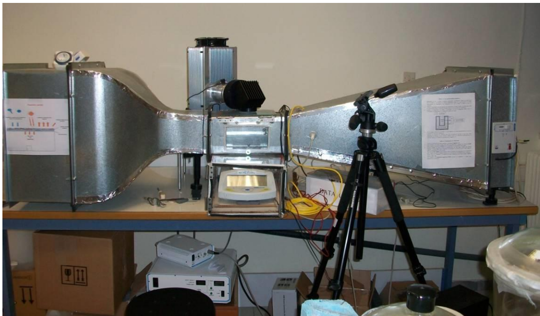
Figure 1: The "wind tunnel" of controllable environmental conditions (Krimpalis and Karamanis. 2015).
