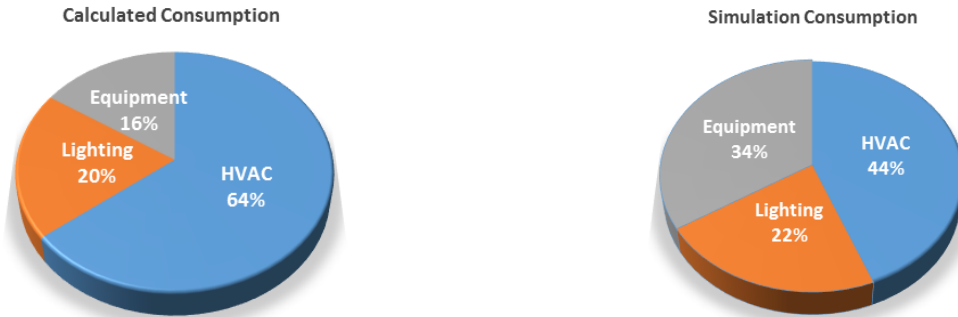
Figure 21: Energy use break down percentage for both methods
