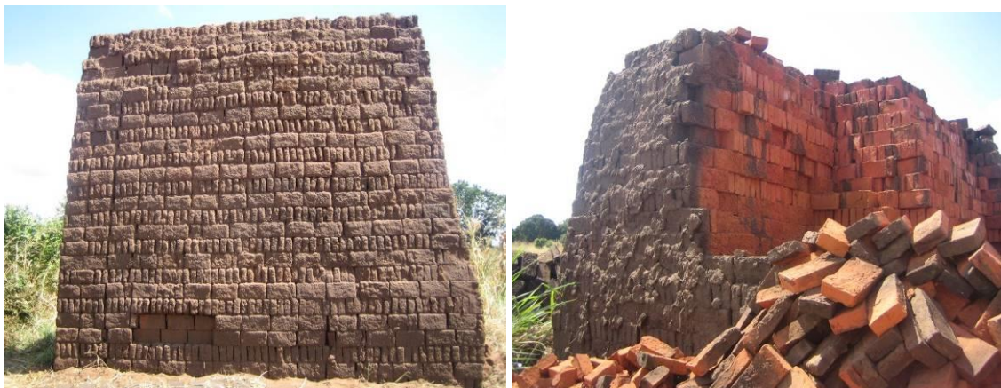
Figure 132: Bricks within 300mm of the clamp kiln's surfaces have a very low quality (Tanzania).
