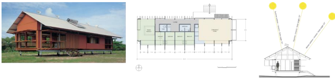
Figure 12. Left: Marika-Alderton house. Photography by: Reiner Blunck. Source: El Croquis (2013). Right: Spatial arrangement and section vs. solar angles. By Authors
