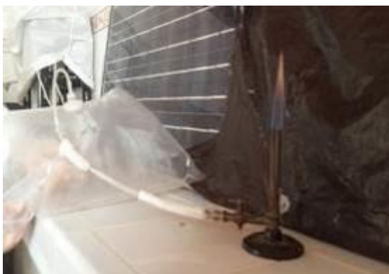
Figure 7: methane flame that confirms the biogas enrichment.
