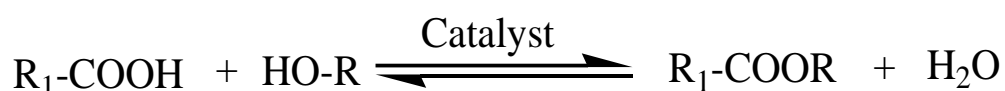
Scheme 1 The esterification of free fatty acid to free acid methyl ester (biodiesel)
