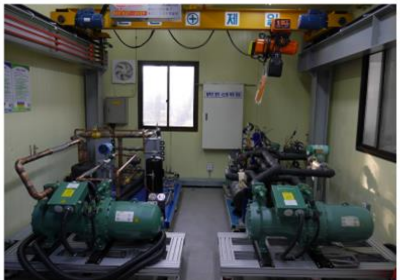
Figure 3. Two paths of discharge bypass cycle and system layout
