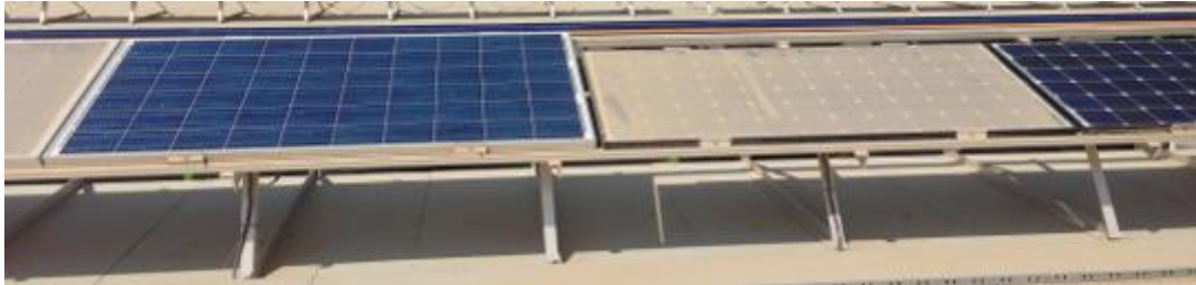
Figure 5: Accumulated dust on PV modules installed in Kuwait, from the left, dusty polycrystalline, clean polycrystalline, dusty monocrystalline and clean monocrystalline.
