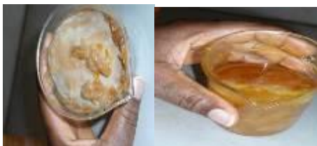
Figure 5: Glycerine obtained when NaOH and KOH were each used as catalysts
