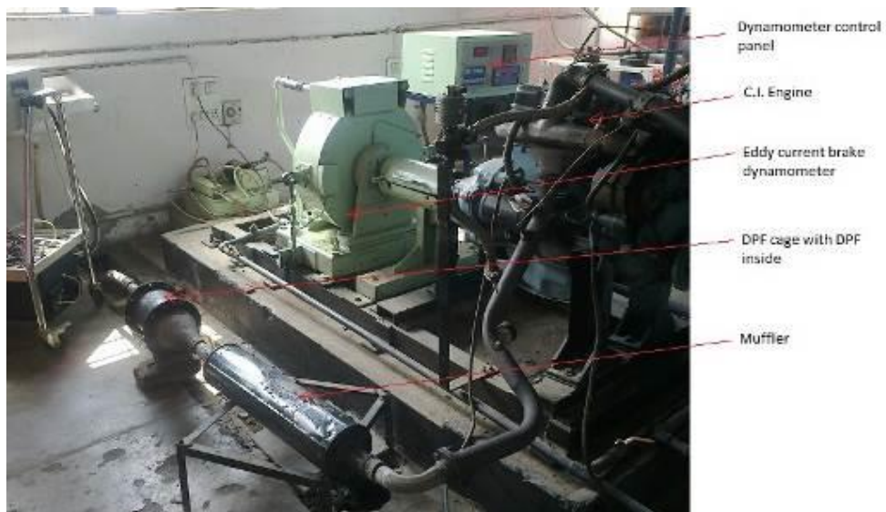
Fig. 2: Laboratory set-up showing the diesel engine, dynamometer, DPF cage, muffler and dynamometer panel.
