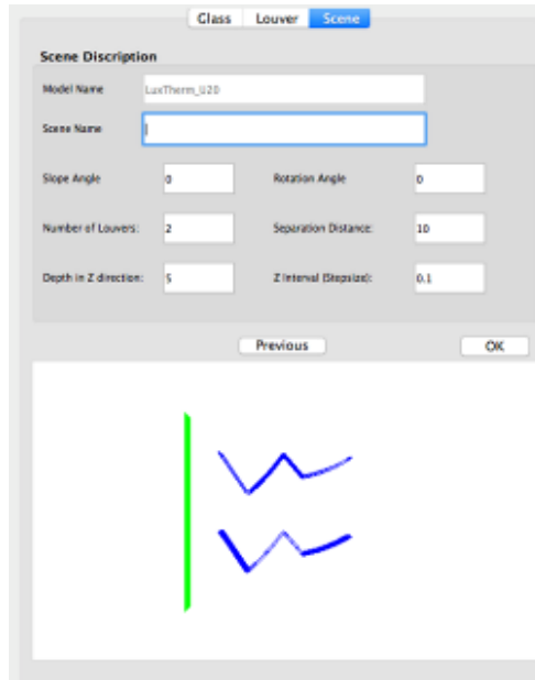
Figure 34: Define a scene that consists of a glass pane and LuxTherm Louvers
