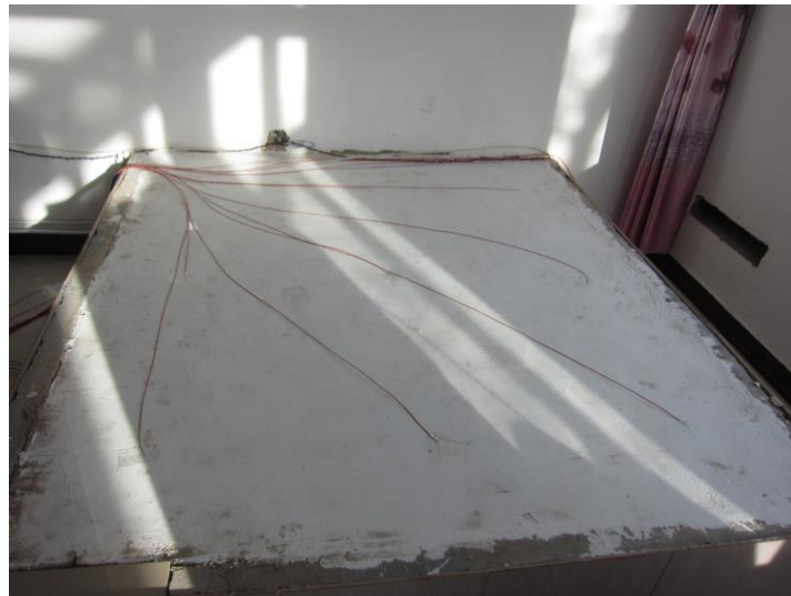
Fig. 3: Thermocouples placed on the surface of Kang body
