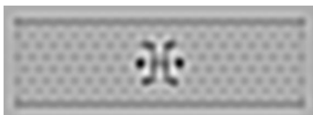
Figure 3s. HRTEM image simulation for a projection of the cluster along the C_3 rotation axis (equivalent to x/y = 45/0 in the tableau above) of [\text{Mo}_6\text{I}_{16}]^{2-} in an armchair (11,11) SWNT.
