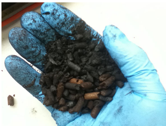
Figure 7. Torrefied pellet extracted from the combustion zone of Power Pallet gasifier after failed experimental run.
