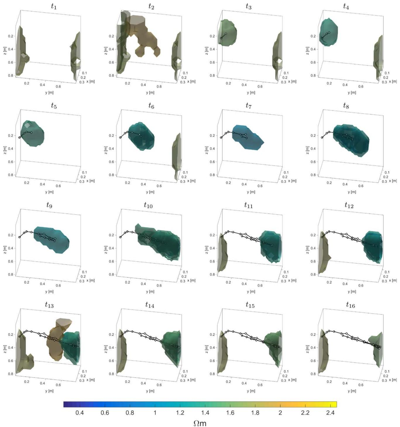
**Figure 8.** Time-slices of 3-D time-lapse ERT model of tank experiment, showing detected MSVs and Kalman filter tracks of the tracked positions up to the current time-slice. MSV surfaces are shaded to represent log mean resistivity.
