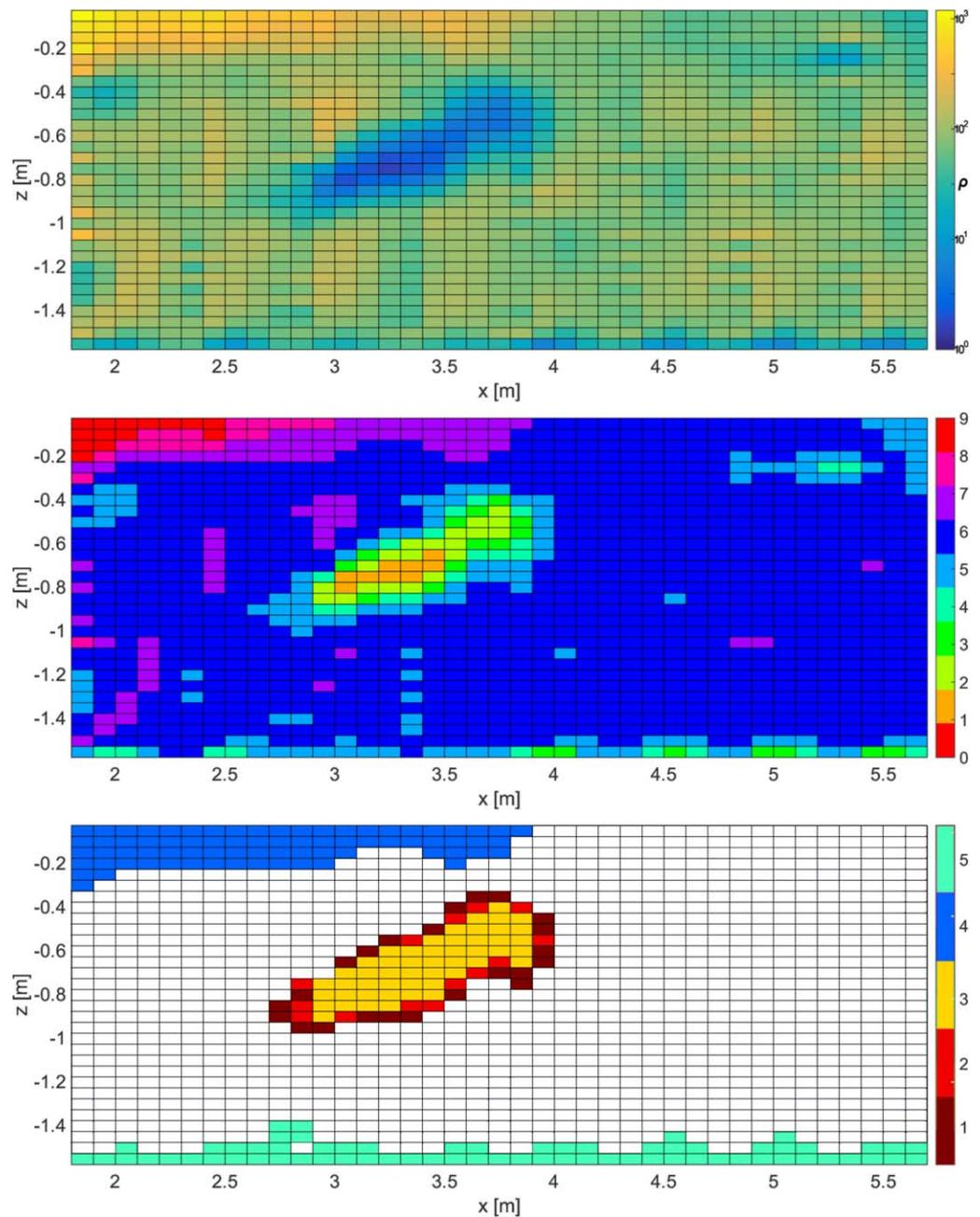
**Figure 3.** 2-D resistivity model of pit experiment at  $t_{20}$ , with results from (middle) distribution-guided fuzzy clustering and (bottom) maximally stable volumes. Individually colored regions represent distinctly separate detected regions which, in the MSV case, exhibit nesting.
