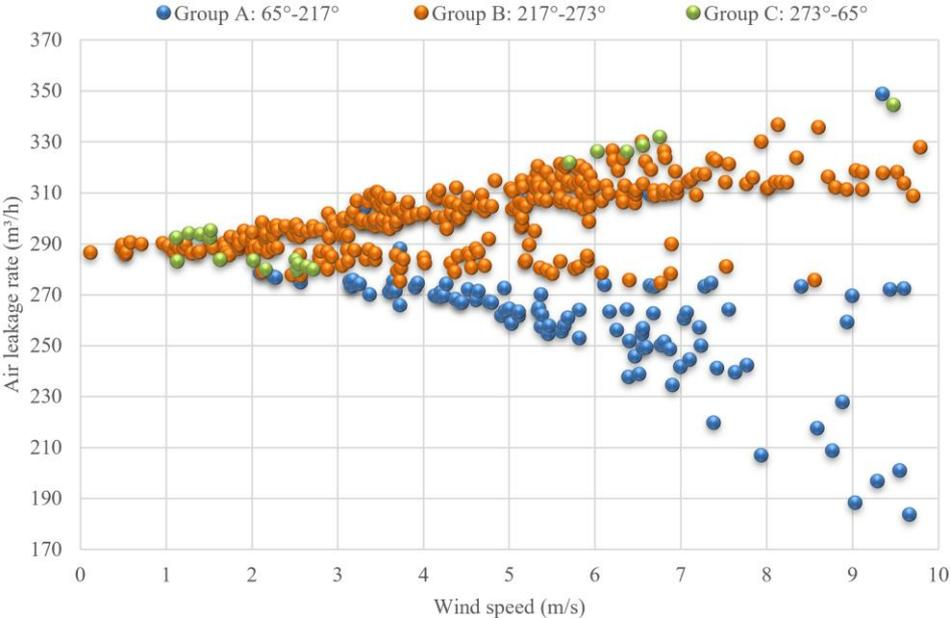
Figure 17: ALR measurements under different wind directions
