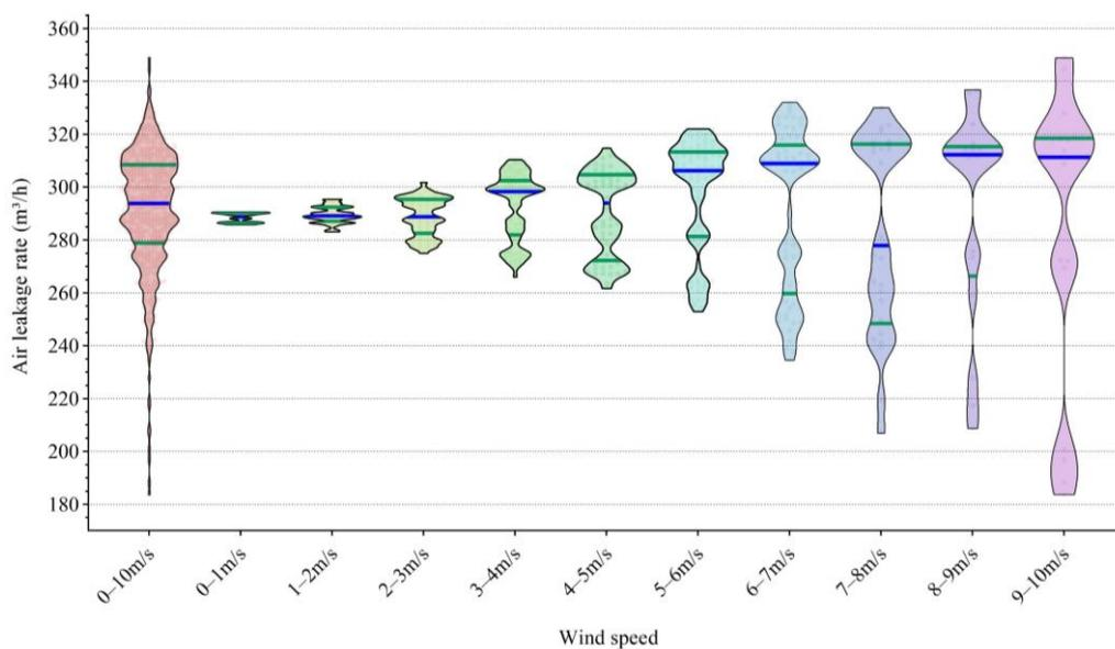
Figure 9: Violin plot of 423 tests
