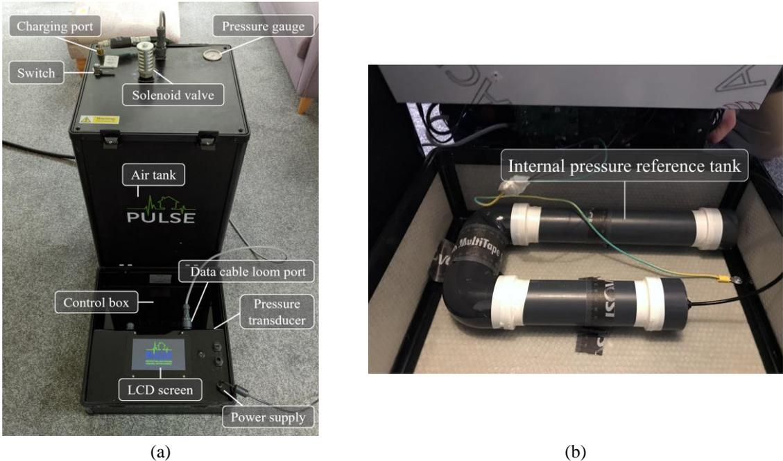
Figure 1: Photos of (a) PULSE-60 unit and (b) internal pressure reference tank of PULSE-60 unit
