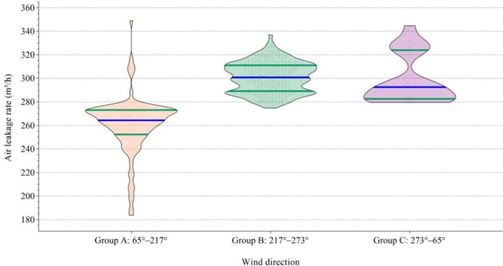
Figure 18: Violin plot of ALR results under different wind directions
