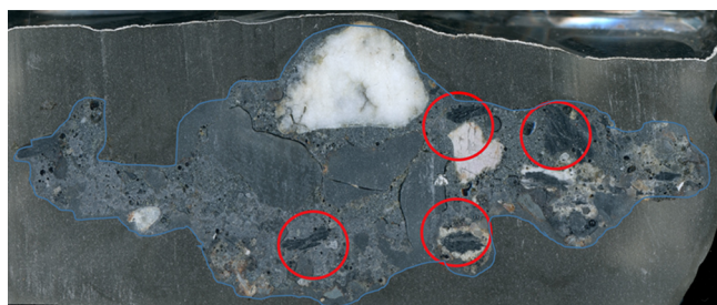
Figure 10. Cross section of ash taken from the Colombian sugar mill stoker furnace. The blue line and shading highlight the outline of the deposit in resin. Red circles highlight the location of carbon-rich lumps encased inside the deposit.
