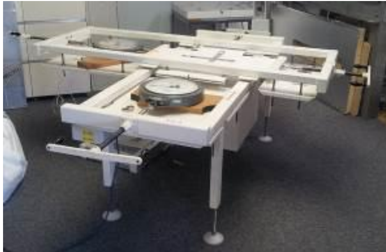
Figure 4: The biaxial machine based on the floating frame concept available at Architen Landrell Associates Limited.
