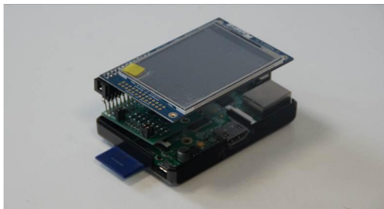
Figure 5: A Raspberry-Pi single-board microcontroller combined with a low cost LCD screen.
