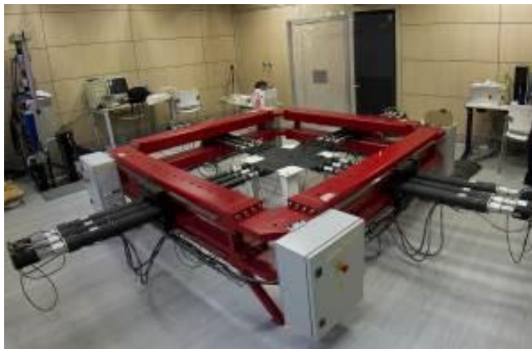
Figure 3: The biaxial machine developed by the author for the clusTEX testing laboratory, Politecnico di Milano.
