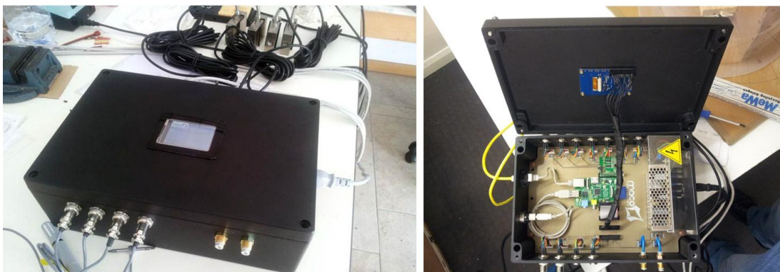
Figure 7: The Raspberry-Pi single-board microcontroller combined with a low cost touchscreen.
