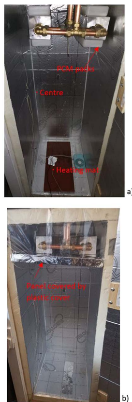
Figure 5. Two test setups: (a) PCM-integrated chilled beam unit, (b) PCM-integrated chilled ceiling panel with a transparent membrane cover.
