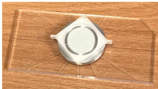
Figure S3: The locating fixture used to image the prepreg using optical microscopy. The prepreg was imaged through the transparent annular region of the smaller acrylic fixture.
