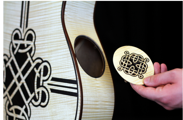
Figure 3: The removable and scannable sound-hole
