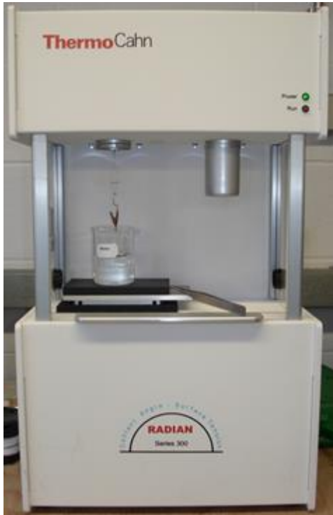
Figure 4. Dynamic contact angle analyser test set-up. A bitumen-coated glass slide hangs (via crocodile clip) from a micro-balance. A movable stage positioned directly below the bitumen-coated slide supports the probe liquid in a glass beaker.
