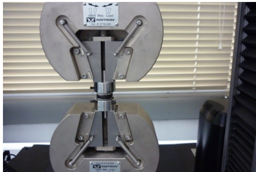
Figure 2. Adhesion strength test set up.
