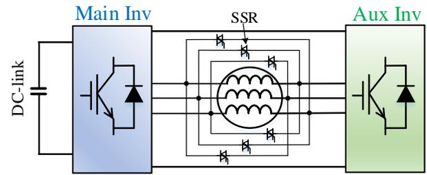
Fig. 18: Reported dual inverter type II structure with the enhanced fault tolerance in [97].
