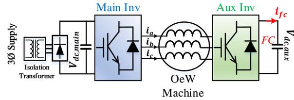
Fig. 16: Dual inverter type III (with a FC).
