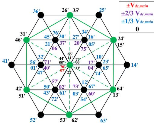
Fig. 15: D-CMV by the dual inverter type II.
