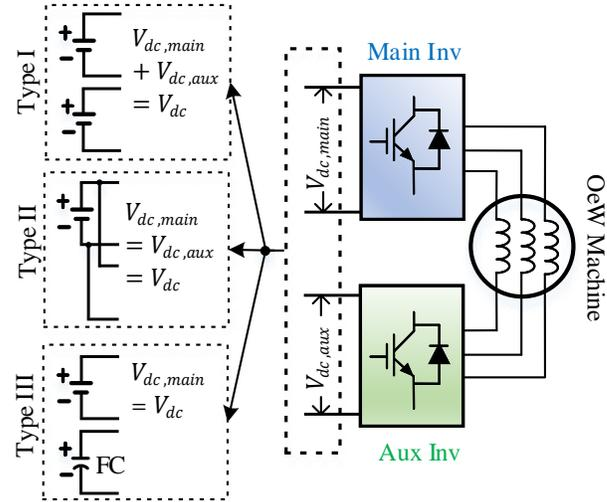
Fig. 4: Three configurations of dual inverter topology.
