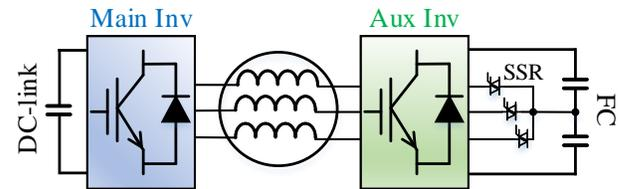
Fig. 19: Reported dual inverter type III structure with the enhanced fault tolerance in [19]–[21].
