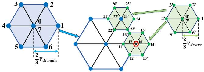
Fig. 3: Space vector diagram by a dual inverter.
