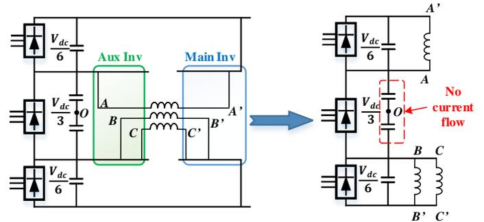
Fig. 13: Motor phases connection for state 11' in the dual inverter with a nested rectifier-inverter.
