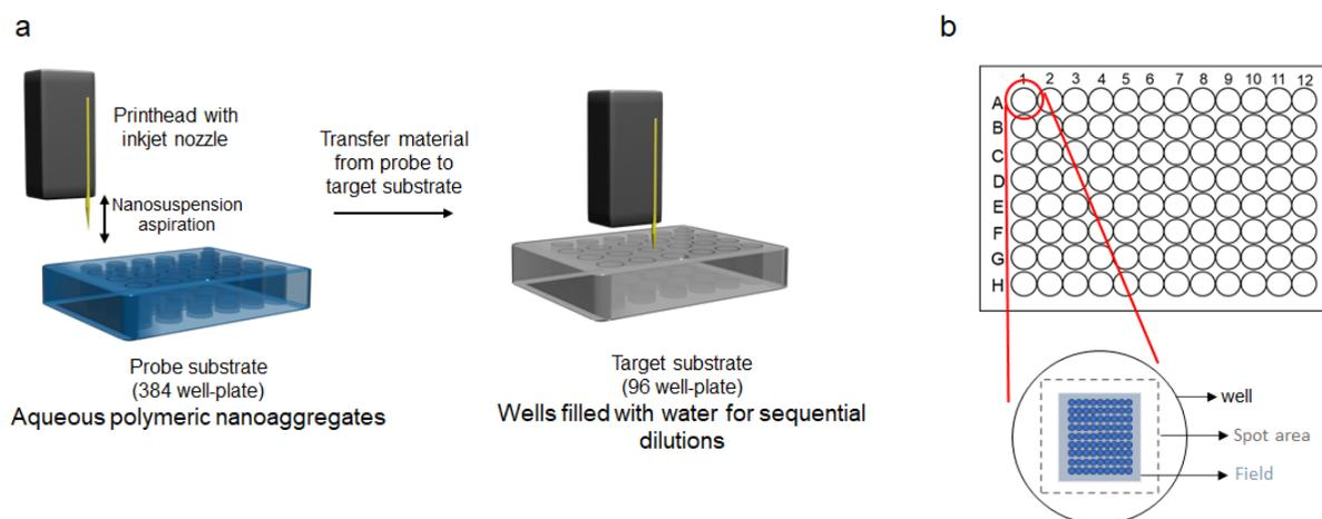
**Figure S2.** (a) Printing process by focusing on the nozzle setup. On the left-hand side, the aqueous polymeric nanosuspension/aggregate aspiration. On the right-hand side, printing dispensing of the aspired nanoaggregates into wells filled with 200  $\mu\text{L}$  of water. (b) the 96-well plate target substrate, detailed view of a well with designed spot area and field, selected print pattern with adjustable number of drops per spot in magnified view.
