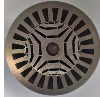
Fig. 8: Photo of stator and rotor cross sections of the prototype, characterised by three flux barriers per pole with central rotor slots to insert the ferrite permanent magnets.
