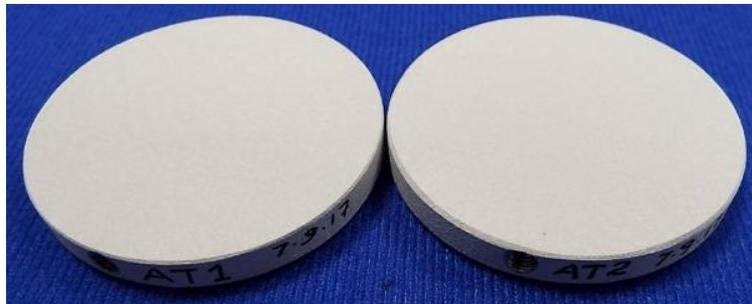
**Figure 4** Representative coupons coated with Keronite's thermal swing coating
