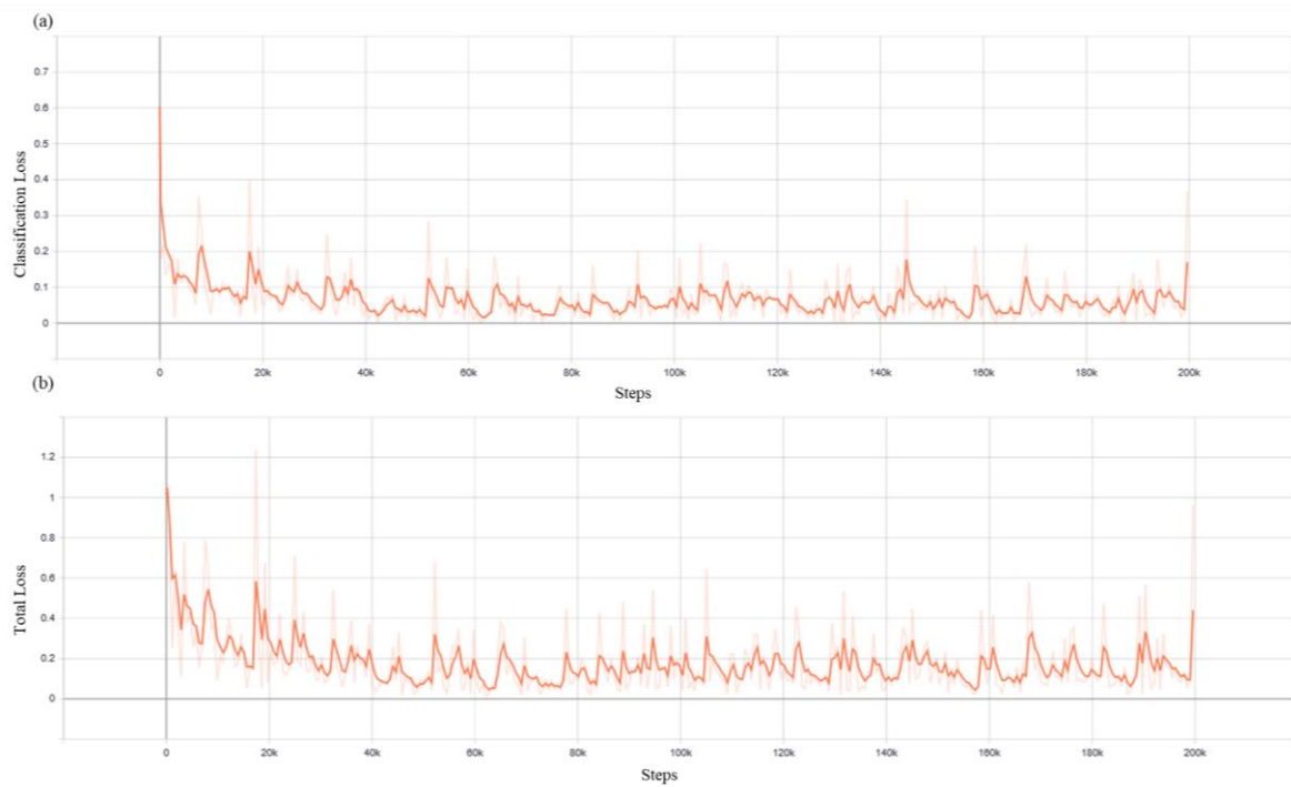
466 467 Figure 9. Training results. (a). Classification loss, and (b). A total loss against the number of training 468 steps.
