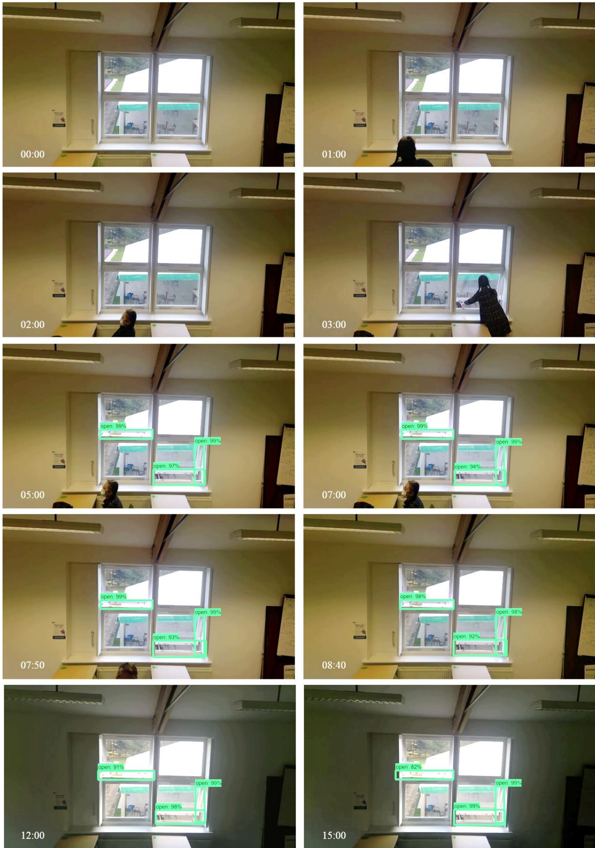
Figure 13. Example snapshots of various key point stages during the application of the window detection approach during Experimental Test 2.
