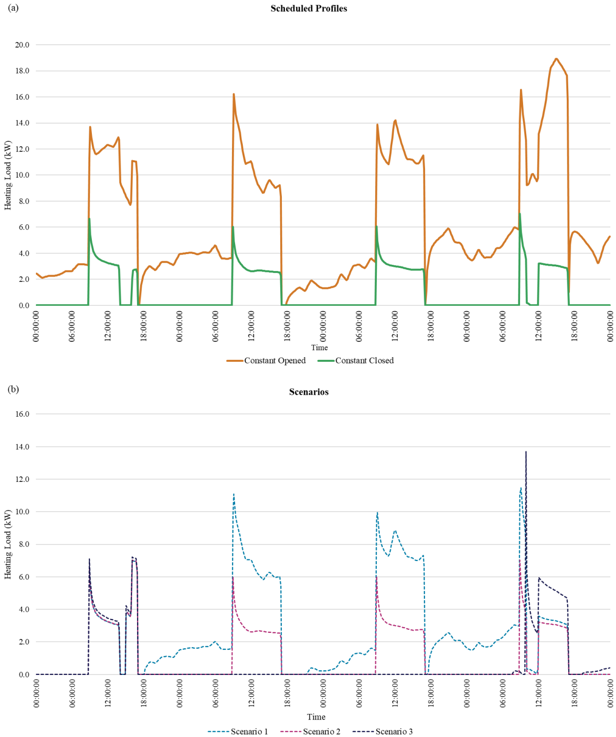
665 Figure 18. Heating load results for a weekend (Friday 10 th – Monday 13 th January) achieved using 666 building energy simulation cases of a). constant scheduled window profiles and b). the three different 667 scenario-based cases.
