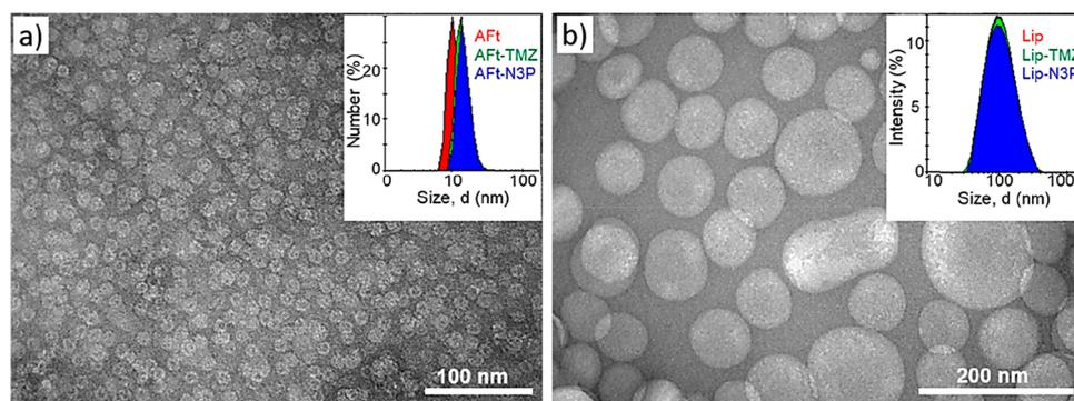
**Figure 1.** Representative TEM images of AFt-N3P ( $\sim 14$  nm) at 160 $\times$  magnification (a) and Lip-N3P ( $\sim 77$  nm) at 87 $\times$  magnification (b). Size distributions measured by DLS are shown in corresponding insets as number frequency curves of control AFt, AFt-TMZ, and AFt-N3P and intensity frequency curves of control Lip, Lip-TMZ, and Lip-N3P at 25 °C in DI water.
