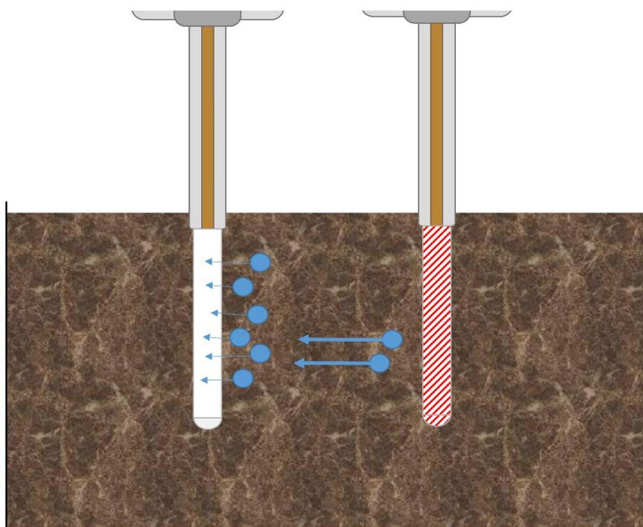
303 **Figure 4.** Diffusion of solutes (blue circles) towards probes implanted in soil matrix. Reduced
