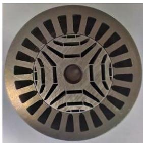
Fig. 12 M1 SynRel prototype front view.
